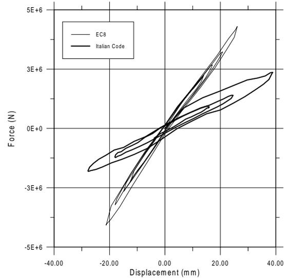
Fig. 13: EC8 and Italian irregular bridge central pier - Free oscillations – Force-Displacement cycles
