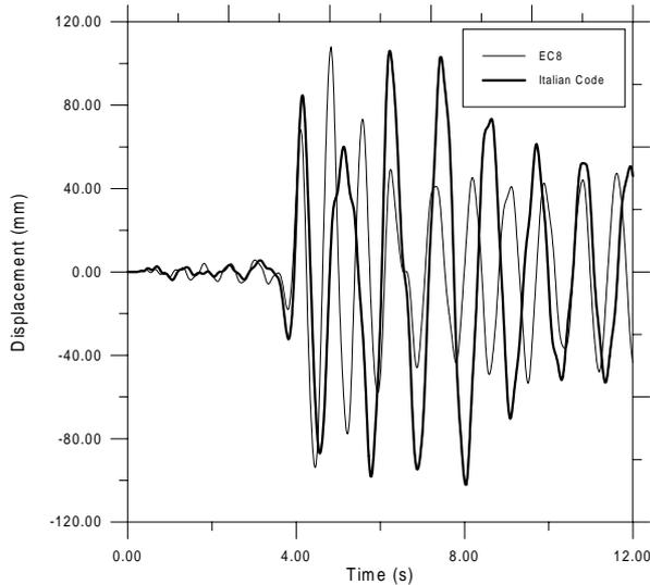
Fig. 14: EC8 and Italian irregular bridge central pier – test with Tolmezzo PGA=0.35g Displacements time history
