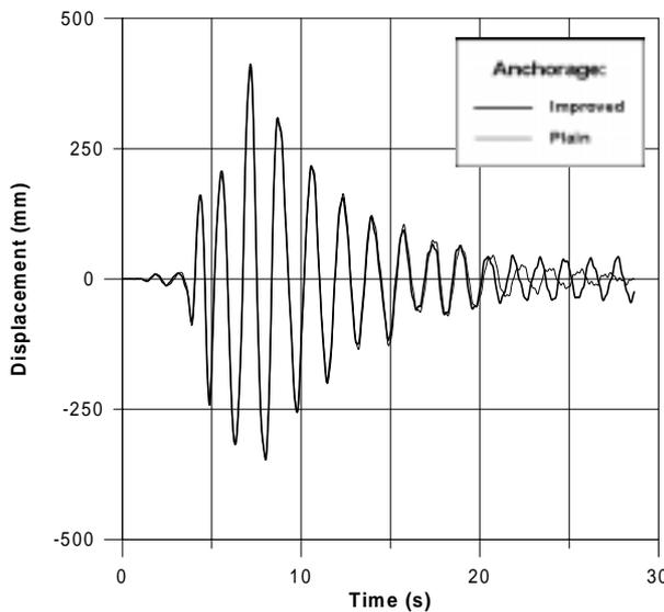
Fig. 10: EC8 regular bridge central pier – Pseudo-dynamic test with Kobe – Displacement time history
