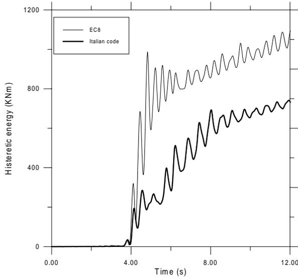
Fig. 16: EC8 and Italian irregular bridge central pier: test with Tolmezzo PGA=0.35g - Dissipated energy time history
