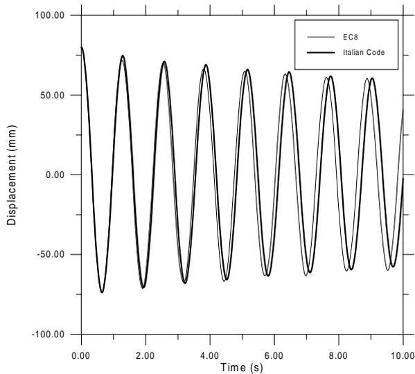
Fig. 18: EC8 and Italian regular bridge lateral pier – free oscillations – Displacements time history
