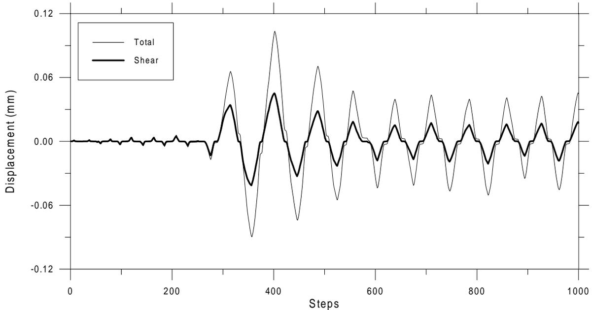
Fig. 9: EC8 irregular bridge central pier with improved anchorage: evaluation of displacements due to shear and flexure.
