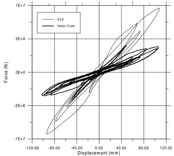
Fig. 15: EC8 and Italian irregular bridge central pier - test with Tolmezzo PGA=0.35g Force-Displacement cycles
