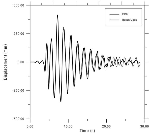
Fig. 19: EC8 and Italian regular bridge lateral pier - pseudodynamic test with Kobe – Displacements time history
