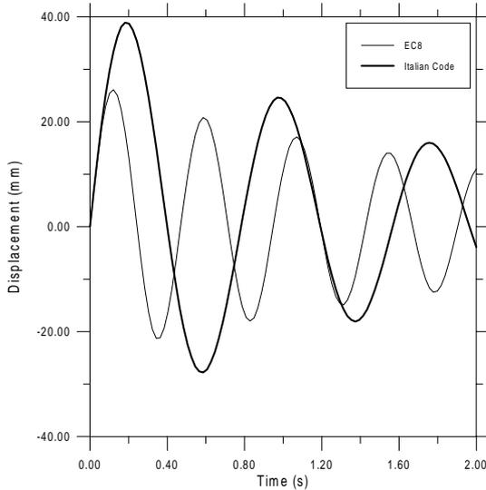
Fig. 12: EC8 and Italian irregular bridge central pier – Free oscillations – Displacement time history
