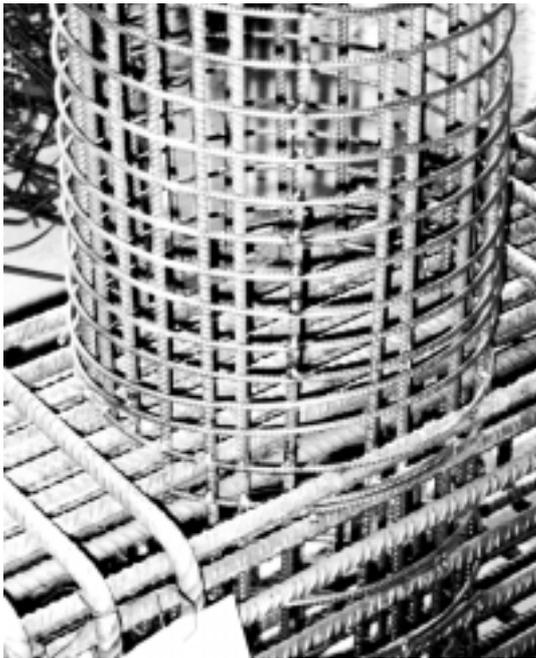
Fig. 3a: EC8 specimen reinforcement detail:
