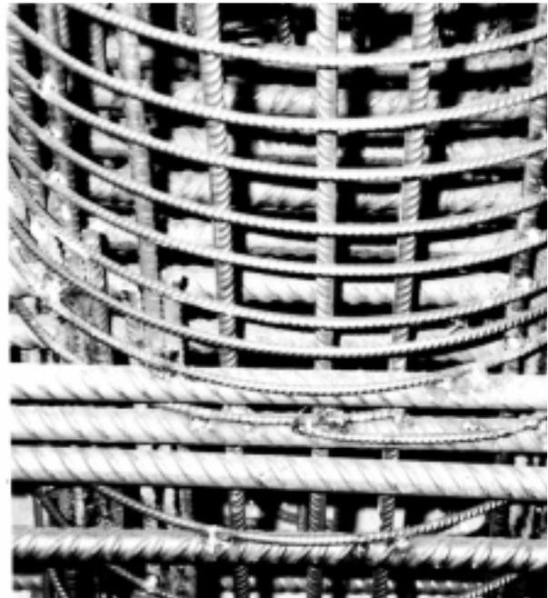
Fig. 3b: EC8 specimen reinforcement detail: improved
