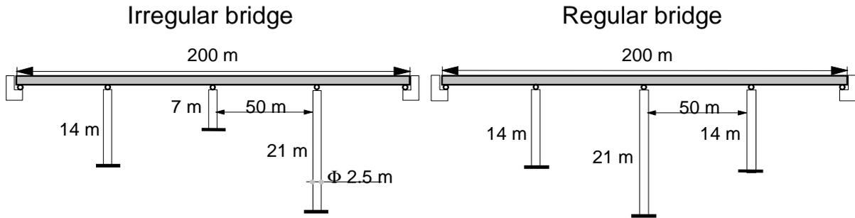
Fig. 1: Layout of designed bridges
