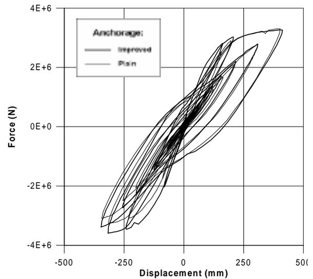
Fig. 11: EC8 regular bridge central pier - Pseudo-dynamic test with Kobe – Force-Displacement cycles
