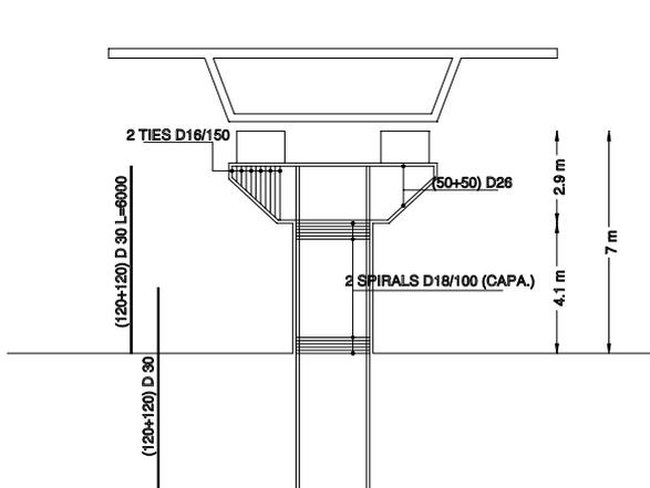
Fig. 2a: EC8 irregular bridge central pier: rebars arrangement (mm)
