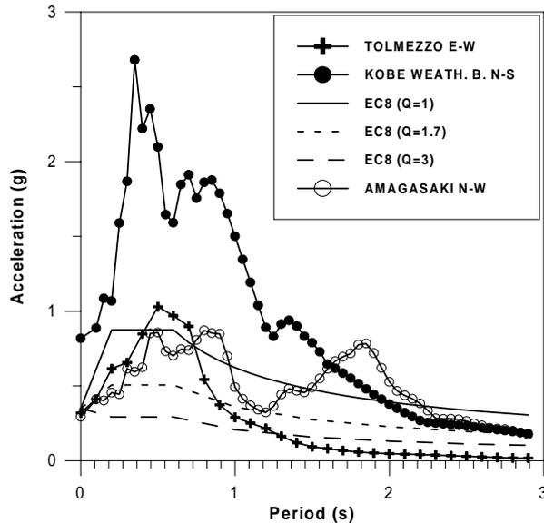
Fig. 4: Natural earthquakes and EC8 spectrum design
