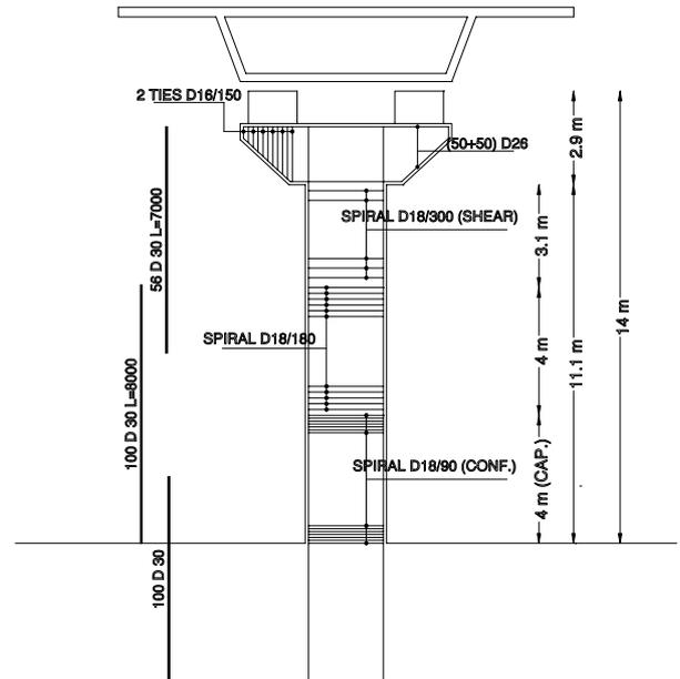
Fig. 2b: EC8 regular bridge lateral pier: rebars arrangement (mm)
