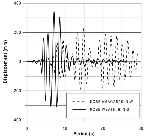
Fig. 5: EC8 regular bridge: numerical simulations response with Kobe earthquake registrations
