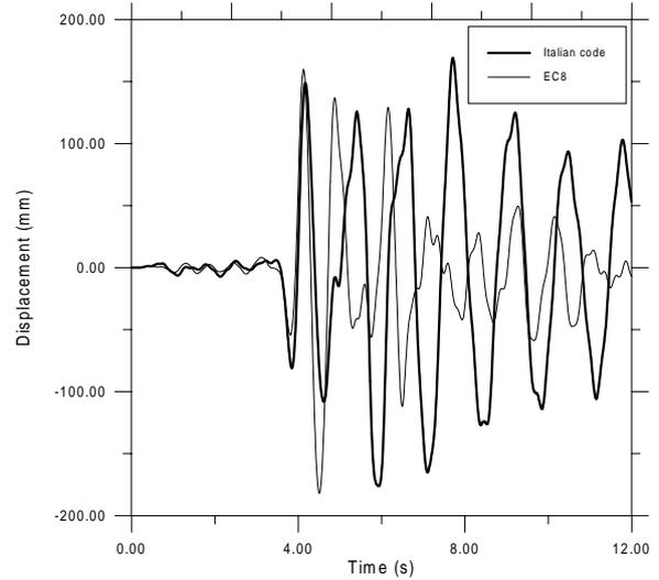
Fig. 17: EC8 and Italian irregular bridge central pier - test with Tolmezzo PGA=0.7g - Displacements time history
