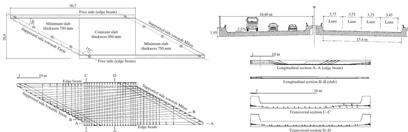
Fig. 1: Slab geometry and prestressing layout
