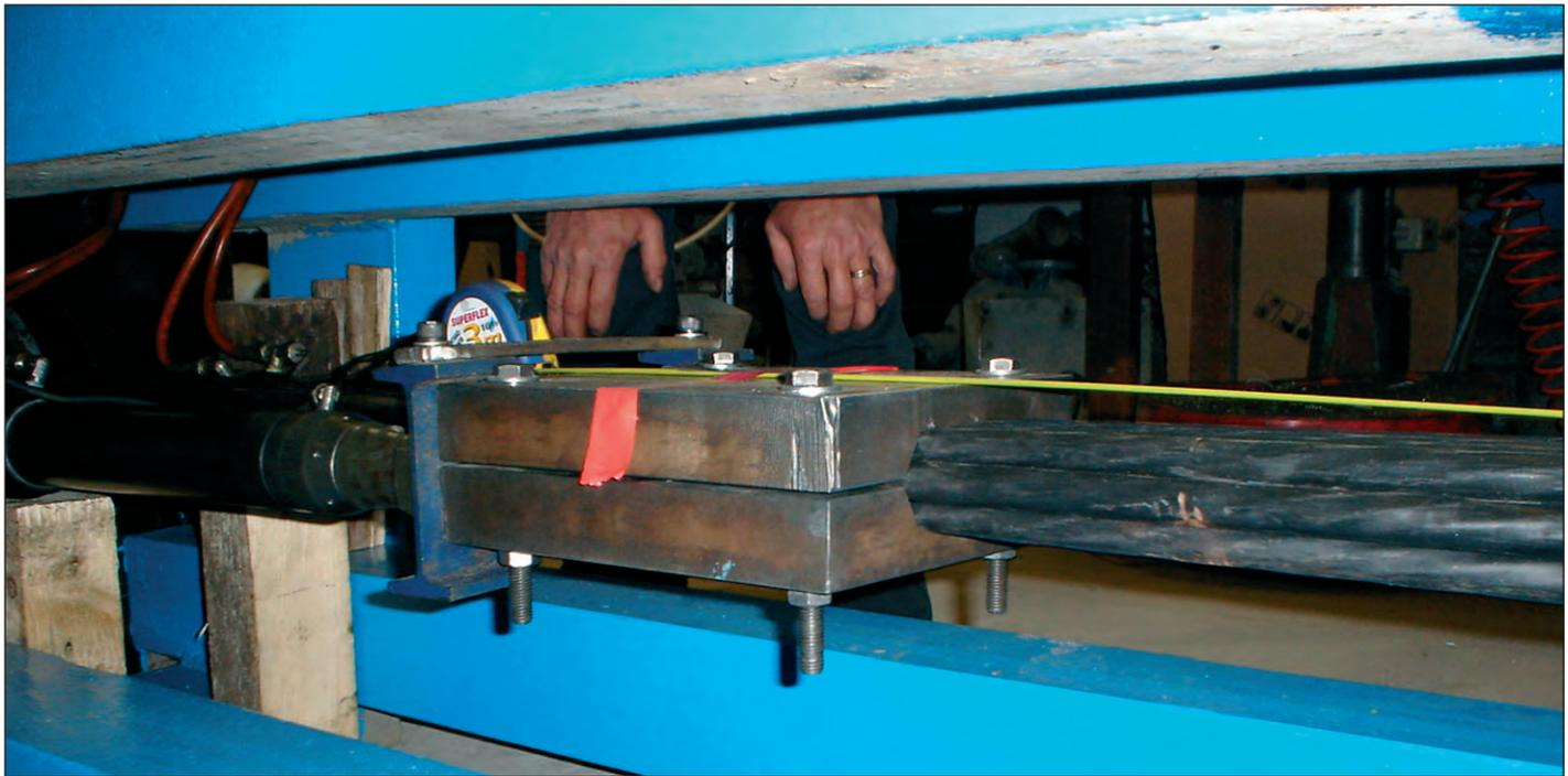
Fig. 8: Test loading of the clamps tangential behaviour
