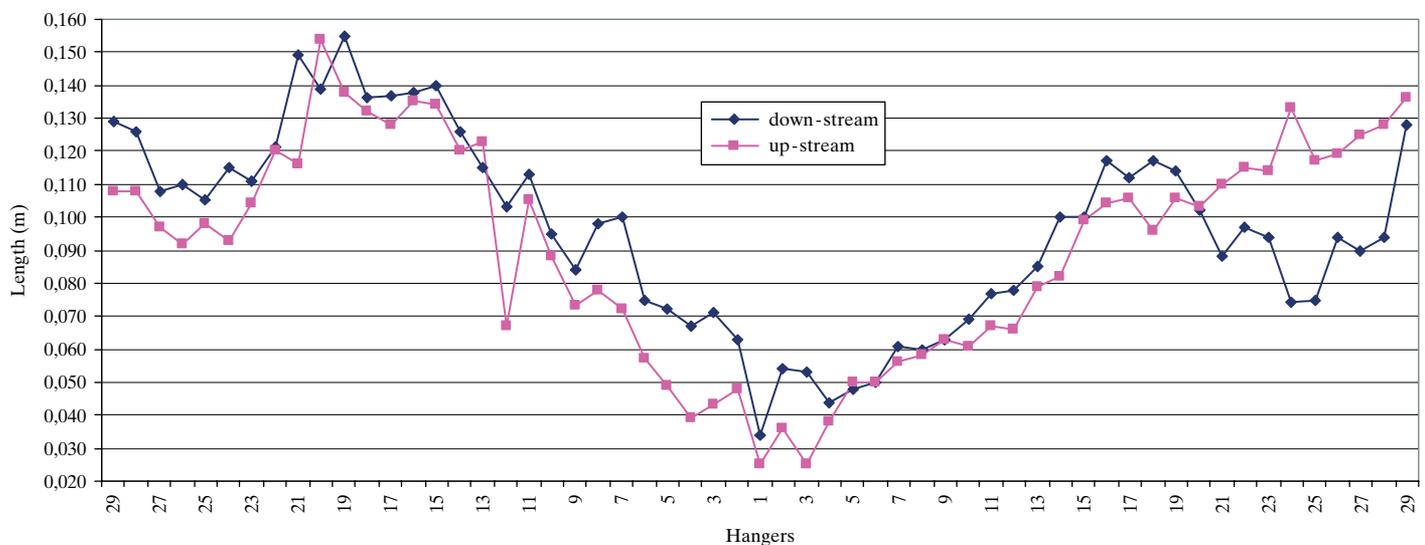
Fig. 13: Hanger's length difference between design and measured value after first tensioning
